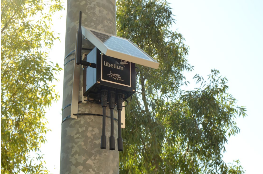
Figure 2: Wasmote Plug & Sense! powered by an external solar panel
