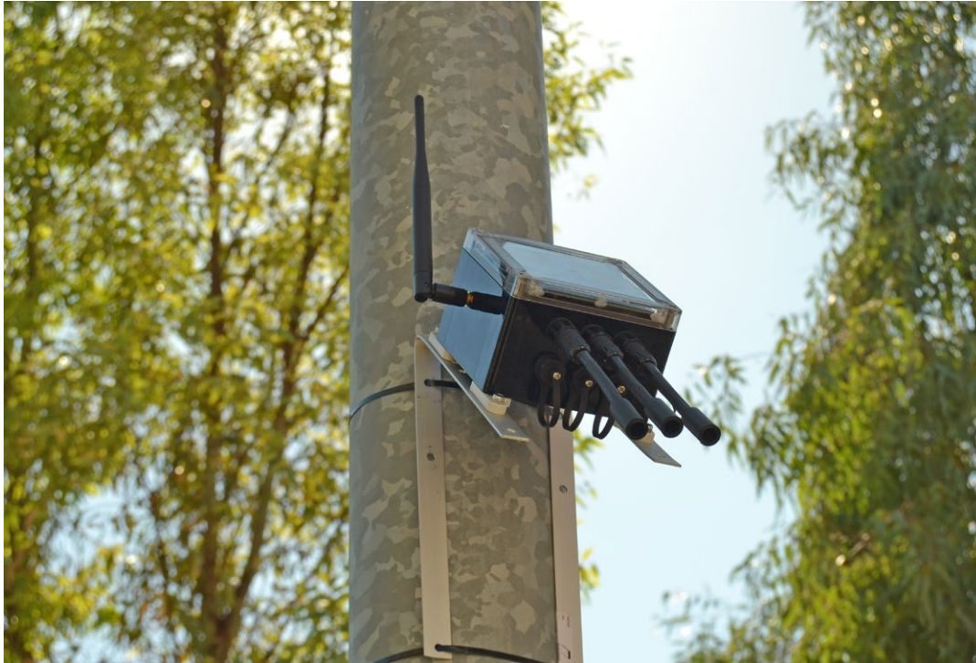
Figure 4: Wasmote Plug & Sense! powered by an internal solar panel
