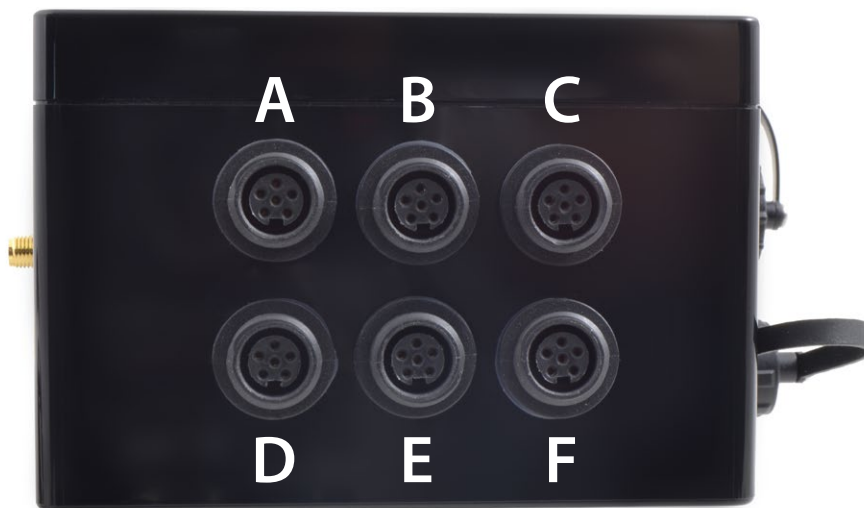
Figure 11: Identification of sensor sockets
