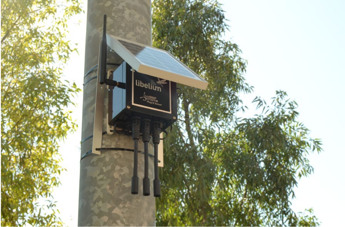
Figure : Waspote Plug & Sense! powered by an external solar panel
