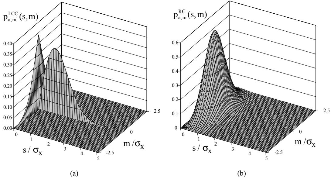
Figure 3: Probability density distributions of counted cycles ( $p_{a,m}^{LCC}$  representation is qualitative since Dirac delta function is not graphicable).
