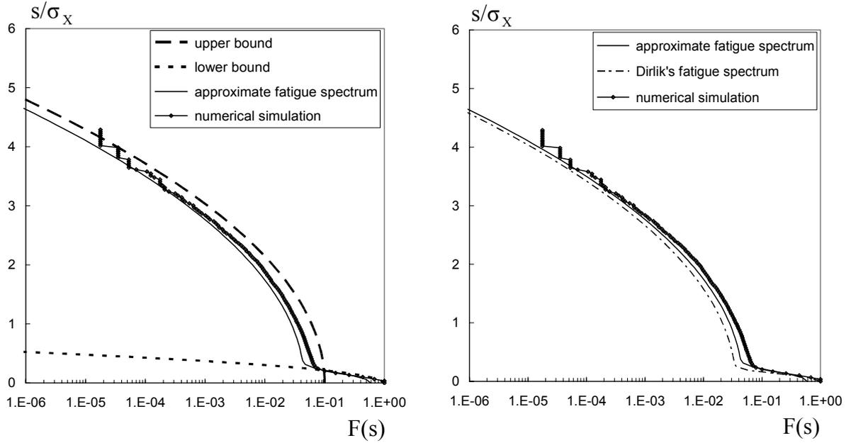
Figure 12: Comparison between numerical fatigue spectra and theoretical estimations (for  $\alpha_2 = 0.1$ ). New method (left); Dirlik's model (right).
