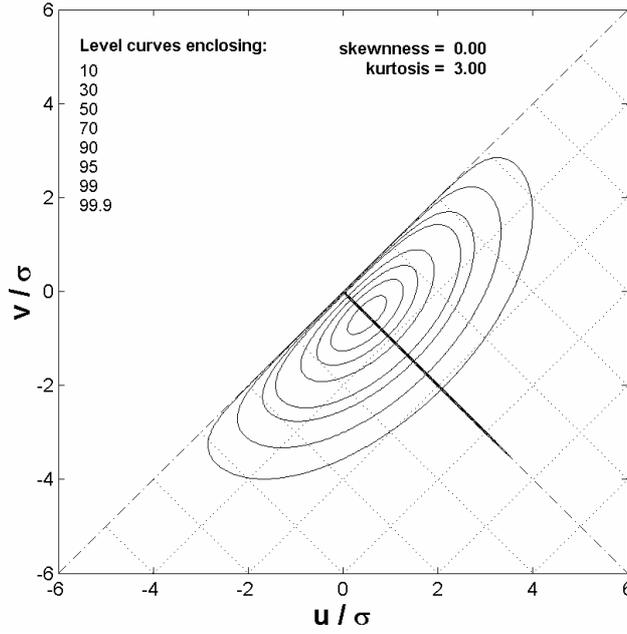
Figure 5: Rainflow cycle distribution  $h_{\text{RFC}}(u, v)$  as a function of peak  $u$  and valley  $v$  levels. Representation of Dirac delta function is qualitative.
