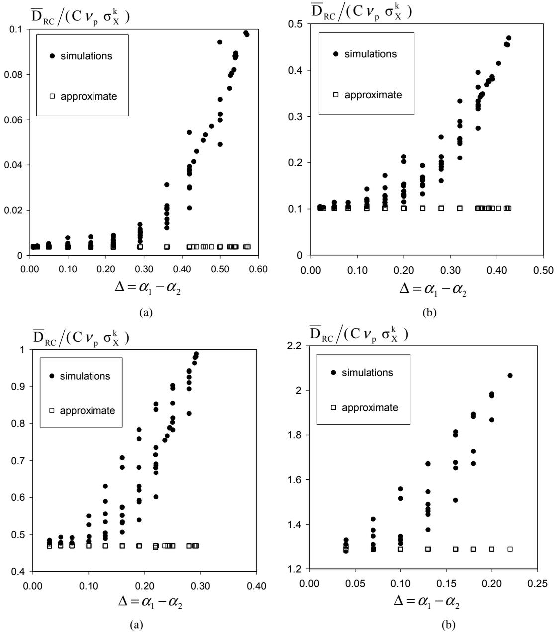
Figure 13: Range-count damage per cycle (slope  $k = 3$ ) obtained from simulations and computed according to approximate formula proposed by Madsen et al. (a)  $\alpha_2 = 0.1$  ; (b)  $\alpha_2 = 0.3$  ; (c)  $\alpha_2 = 0.5$  ; (d)  $\alpha_2 = 0.7$  .
