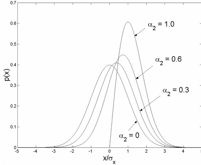
Figure 2: Probability density of peaks,  $p_p(x)$ , for different values of  $\alpha_2$  parameter.
