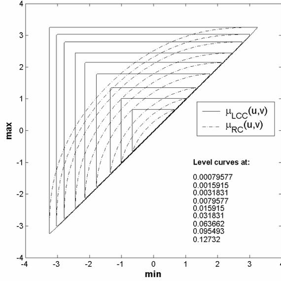
Figure 4: Comparison of  $\mu_{LCC}(u, v)$  and  $\mu_{RC}(u, v)$  count intensities for a Gaussian process with  $\lambda_0 = \lambda_2 = 1$  and  $\lambda_4 = 4$  ( $\alpha_2 = 0.5$ ).
