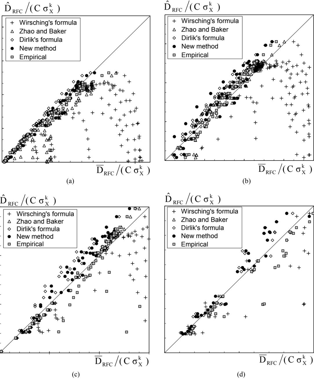
Figure 11: Comparison of damages for processes having different irregularity factors. Slope  $k = 5$ . (a)  $\alpha_2 = 0.1$  ; (b)  $\alpha_2 = 0.3$  ; (c)  $\alpha_2 = 0.5$  ; (d)  $\alpha_2 = 0.7$  .
