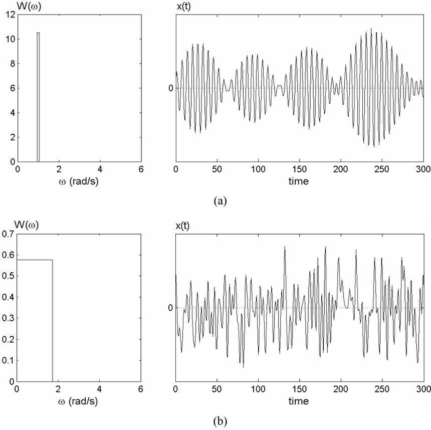
Figure 1: Examples of (a) narrow-band and (b) broad-band process.
