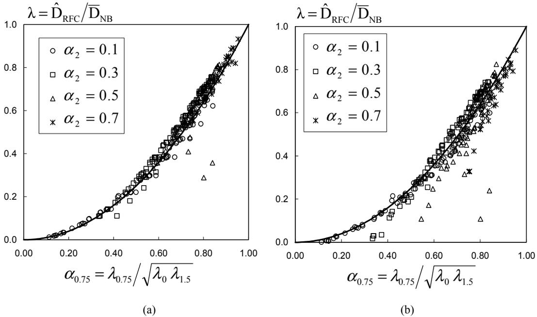
Figure 9: Relationship between  $\alpha_{0.75}$  and  $\lambda_{BT}$  correction factor. The expression  $\lambda_{BT} = \alpha_{0.75}^2$  (continuous line) is compared with simulations (dots). S-N slope (a)  $k = 3$  and (b)  $k = 5$ .
