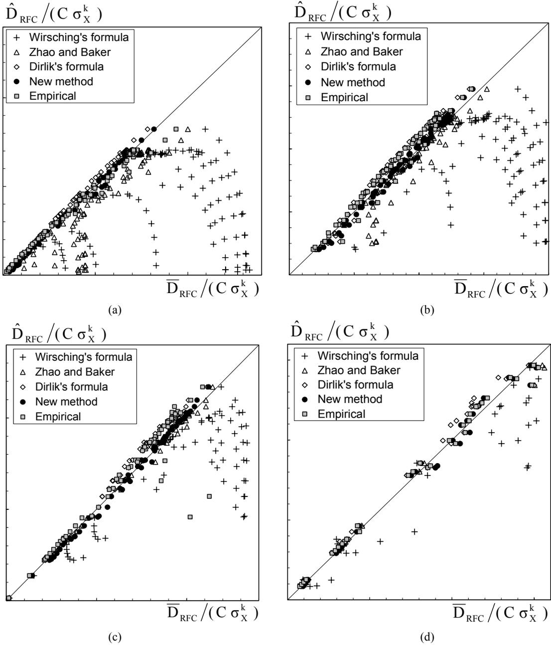
Figure 10: Comparison of damages for processes having different irregularity factors. Slope  $k = 3$ . (a)  $\alpha_2 = 0.1$  ; (b)  $\alpha_2 = 0.3$  ; (c)  $\alpha_2 = 0.5$  ; (d)  $\alpha_2 = 0.7$  .
