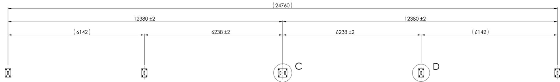
REQUIRED POSITION AND SPACING OF THE CONCRETE FOOTINGS AND STAND CENTRELINES
