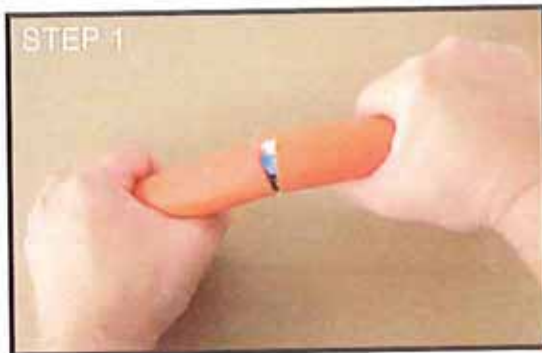
STEP 1 Cut all around and bend the jacket to ensure a complete cut.
