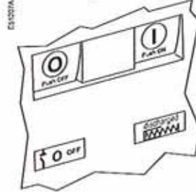
Circuit breaker open and discharged
