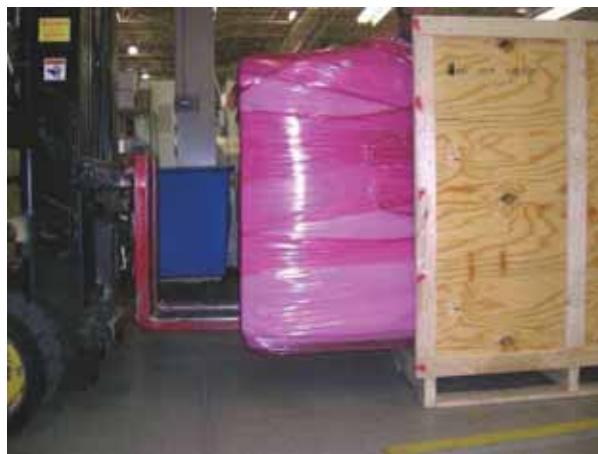
Figure 6 Removing Unit from Crate with Forklift
